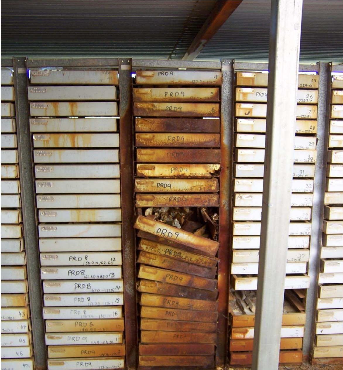
Core samples from the Peak Hill gold mine's sulfide zone left to their own devices (water and air). The DZP's most expensive input will be sulfuric acid, which this deposit may provide, complete with a gold byproduct offset.
